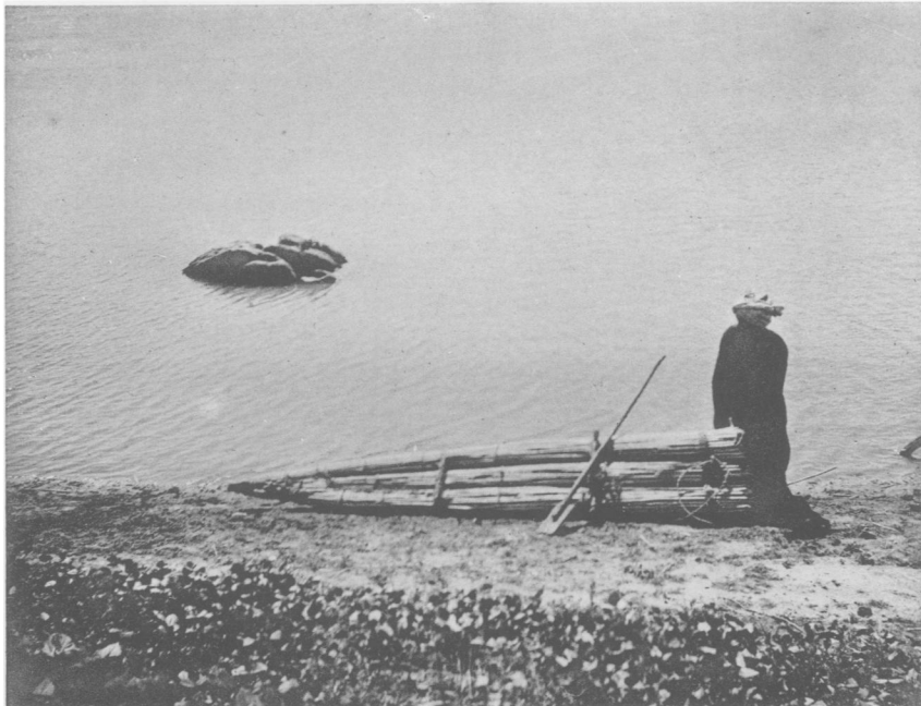
Fig. 2. A NUBIAN REED-FLOAT AT TOMBOS, SHOWING HOW THE TRIPLE BUNDLES ARE LASHED TOGETHER
